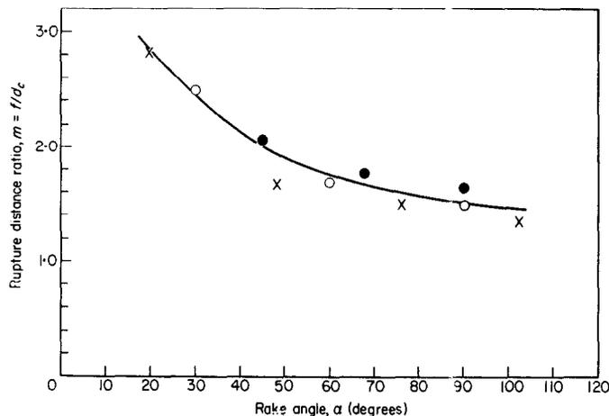
Fig. 11. Experimental relationship between rupture distance ratio and tine rake angle. ●, From Fig. 3; ○, from Hettiaratchi and Reece<sup>6</sup>; ×, from Payne<sup>4</sup> and Payne and Tanner<sup>11</sup>
