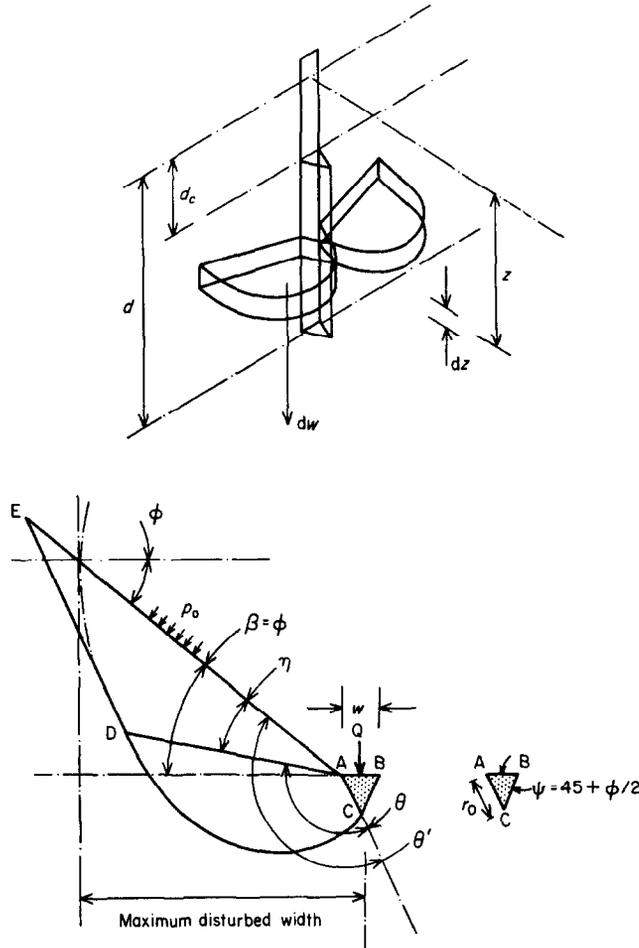
Fig. 7. Lateral soil failure mechanism
