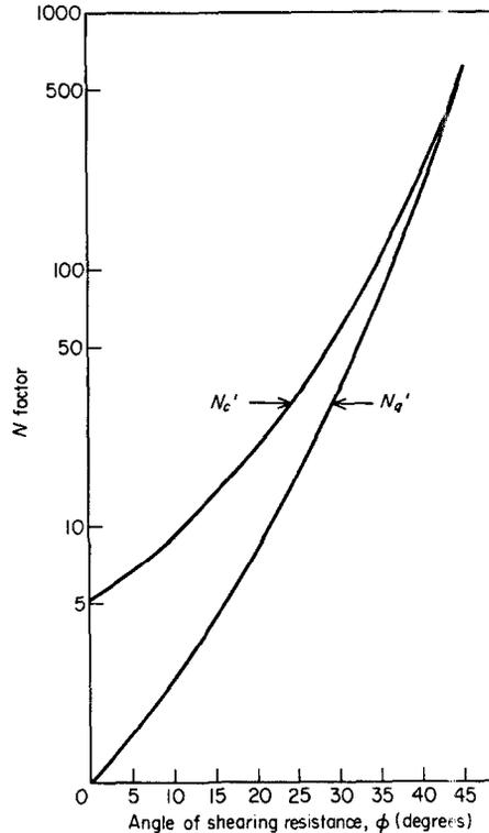
Fig. 8. Dimensionless  $N$  factors for lateral soil failure
