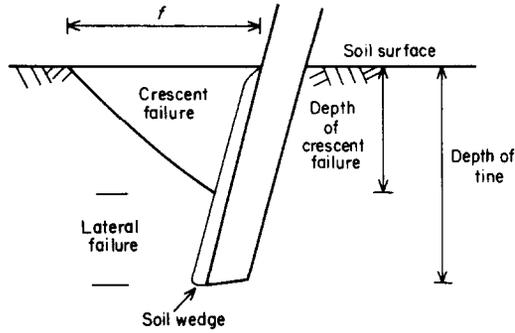
Fig. 1. Soil failure pattern
