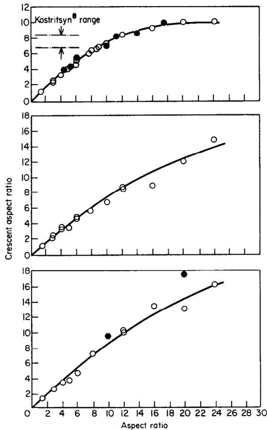
Fig. 2. Relationship between crescent aspect ratio and aspect ratio for 90° rake angle tines (top), 67.5° rake angle tines (middle) and 45° rake angle tines (bottom). Solid points from Miller<sup>9</sup>
