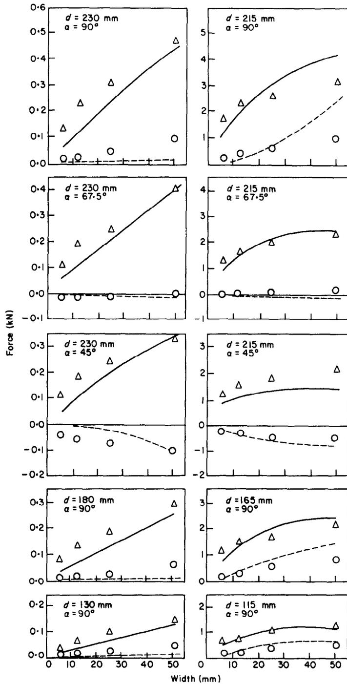
Fig. 12. Comparison between predicted and measured forces for a range of tine widths, in uncompacted soil (left) and compacted soil (right). —, Predicted horizontal force; ---, predicted vertical force;  $\Delta$ , measured horizontal force;  $\circ$ , measured vertical force
