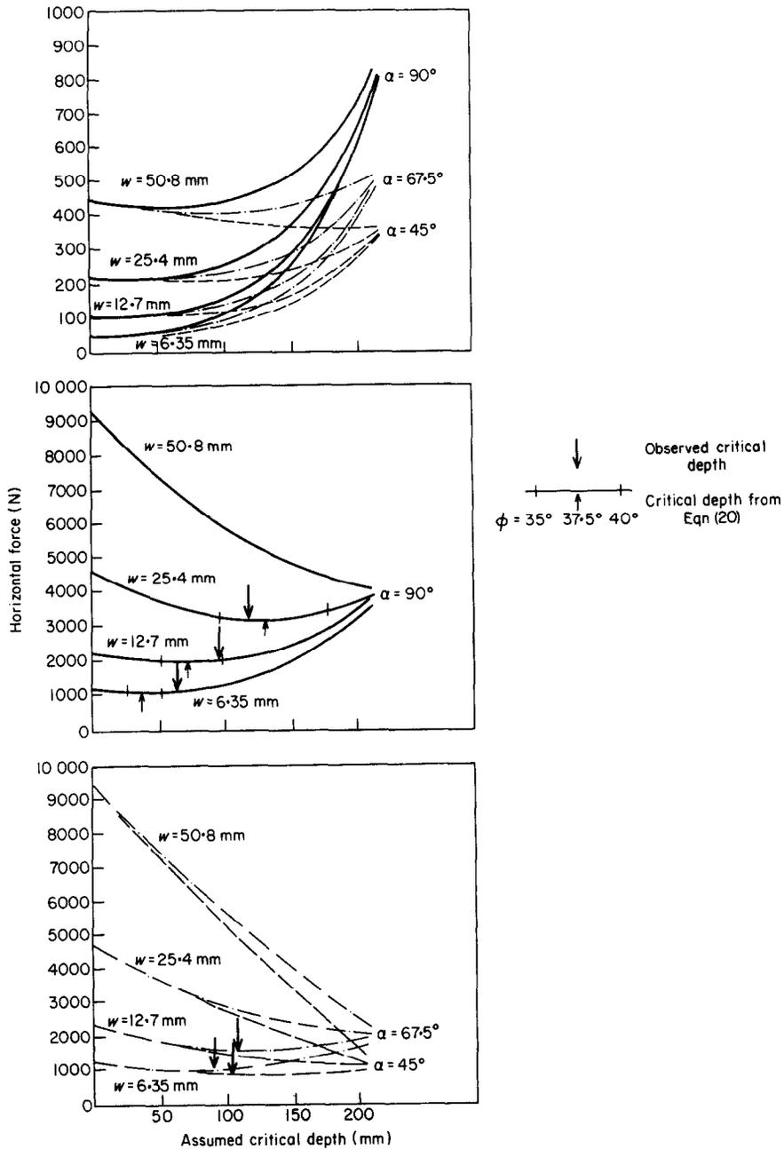
Fig. 10. Relationship between the horizontal force and the position of the assumed critical depth. Top:  $90^\circ$ ,  $67.5^\circ$  and  $45^\circ$  rake angles, uncompact soil. Middle:  $90^\circ$  rake angle, compacted soil. Lower:  $67.5^\circ$  and  $45^\circ$  rake angles, compact soil
