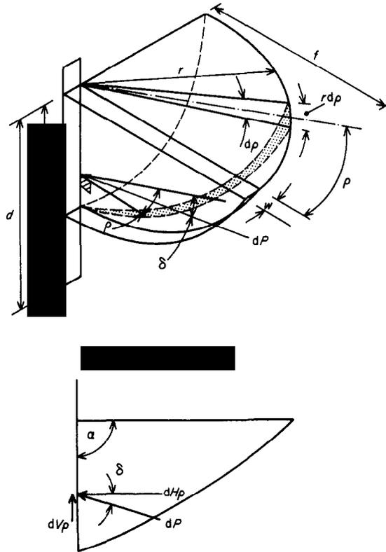
Fig. 6. Crescent soil failure mechanism
