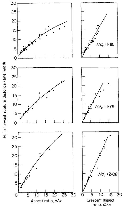
Fig. 3. Left: relationship between the ratio of forward rupture distance/tine width and aspect ratio for 90° rake angle tines (top), 67.5° rake angle tines (middle) and 45° rake angle tines (bottom). Crosses from Payne<sup>4</sup> and Payne and Tanner.<sup>11</sup> Right: relationship between the ratio of forward rupture distance/tine width and crescent aspect ratio for 90° rake angle tines (top) 67.5° rake angle tines (middle) and 45° rake angle tines (bottom)
