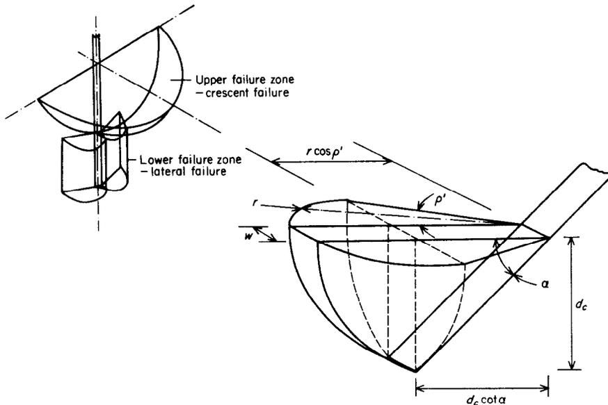
Fig. 5. Left: conceptual mechanism of soil failure. Right: crescent geometry
