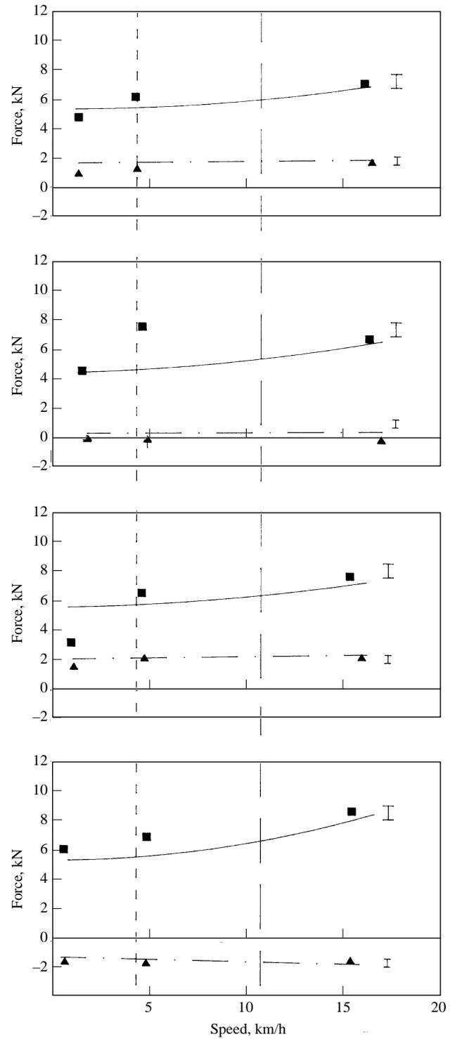
Fig. 8. Effect of speed on forces acting on a single tine with rake angle of 30° (top), 40° (upper centre), 60° (lower centre) and 90° (bottom) in cohesive soil. Also shown are the l.s.d. bands at 0.05 probability level for the experimental data. ■, Measured horizontal force component; ▲, measured vertical force component; —, predicted horizontal force component; - - -, predicted vertical force component
