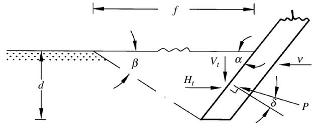
Fig. 1. Wide tine showing soil failure plane
