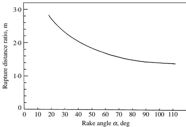
Fig. 3. Experimental relationship between rupture distance ratio ( $m = f/d$ ) and tine rake angle ( $\alpha$ ) (after Godwin and Spoor<sup>3</sup>)
