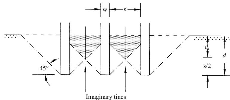
Fig. 6. Front view of triple tine arrangement showing imaginary tines
