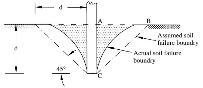
Fig. 4. Cross-section of typical tine failure soil profile
