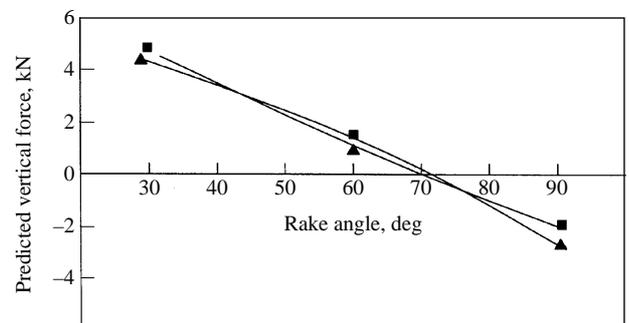
Fig. 2. Comparison of vertical force predictions from original (■) and simplified (▲) equations for a 0.03 m wide tine at 0.25 m depth in soil with  $\phi = 30^\circ$ ,  $c = 30 \text{ kN/m}^2$  and  $\delta = 20^\circ$
