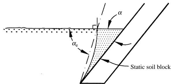
Fig. 5. Non-scouring (static) soil block on tine face
