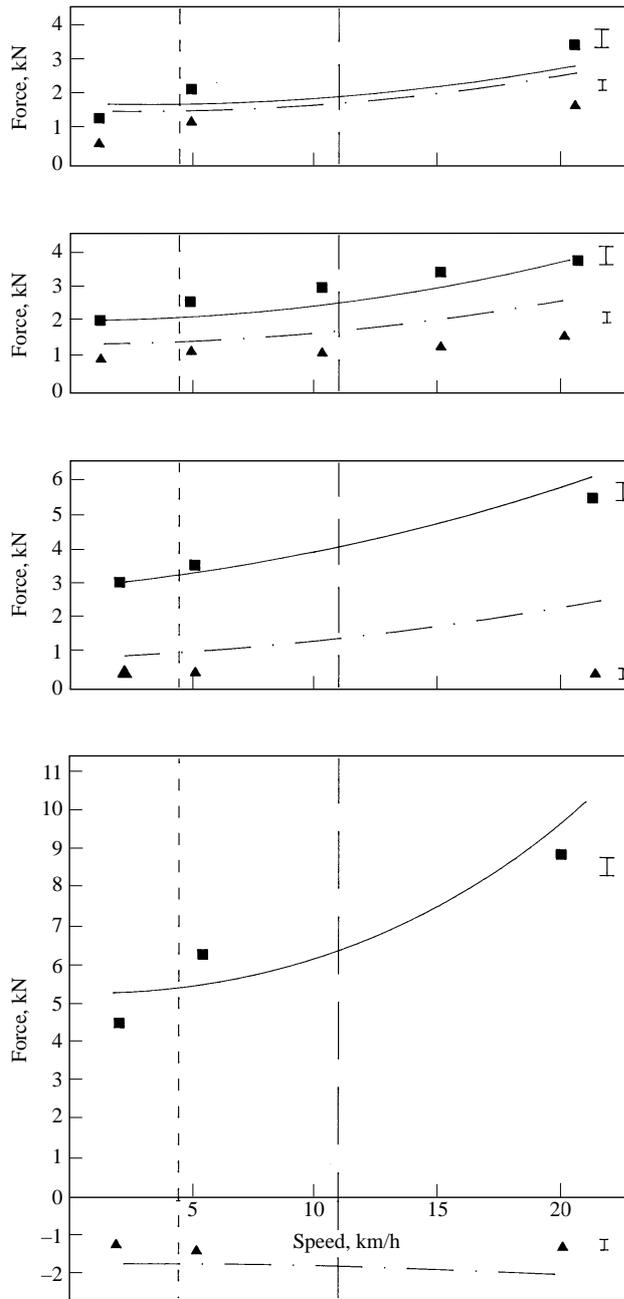
Fig. 7. Effect of speed on forces acting on a single tine with rake angle of 30° (top), 40° (upper centre), 60° (lower centre), and 90° (bottom) in frictional soil. Also shown are the l.s.d. bands at 0.05 probability level for the experimental data. ■, Measured horizontal force component; ▲, measured vertical force component; —, predicted horizontal force component; - - -, predicted vertical force component
