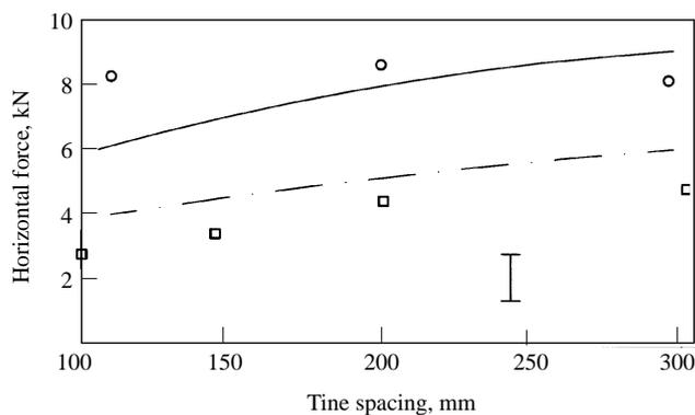
Fig. 9. The effect of tine spacing and speed on horizontal force component acting on multiple tines with a rake angle of  $40^\circ$  in frictional (laboratory) soils at two speeds. Also shown with the l.s.d. band at 0.05 probability level for the experimental data.  $\circ$ , Measured 20 km/h;  $\square$ , measured 5 km/h; —, predicted 20 km/h; - - -, predicted 5 km/h
