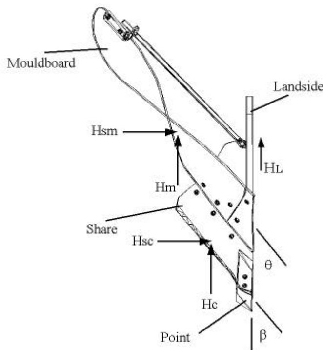
Figure 1. Diagram of the mouldboard forces.
