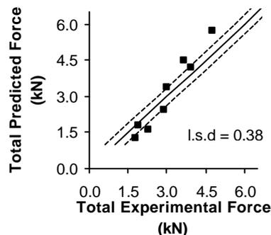
**Figure 4. A comparison of experimental and predicted total draught forces.**
