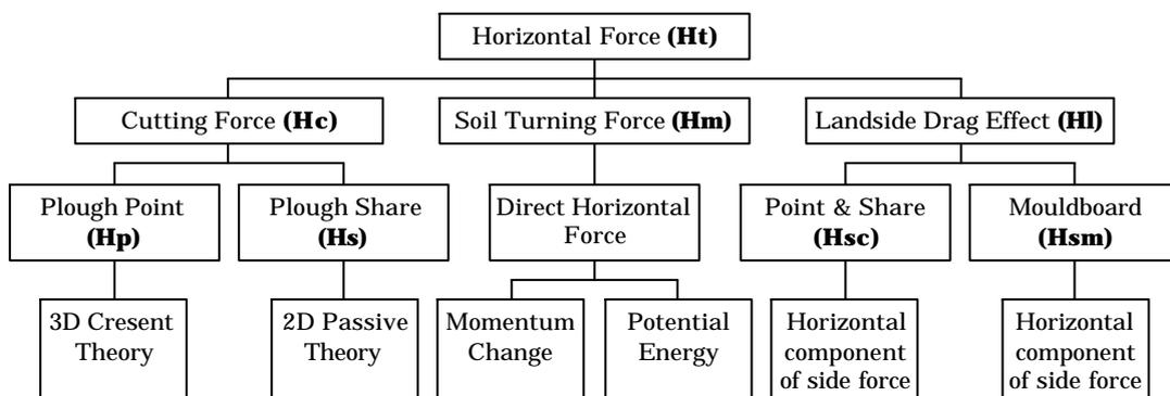
Figure 2. Force components acting on a mouldboard plough.
