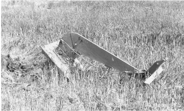
Fig. 1. Soil anchor used in study
