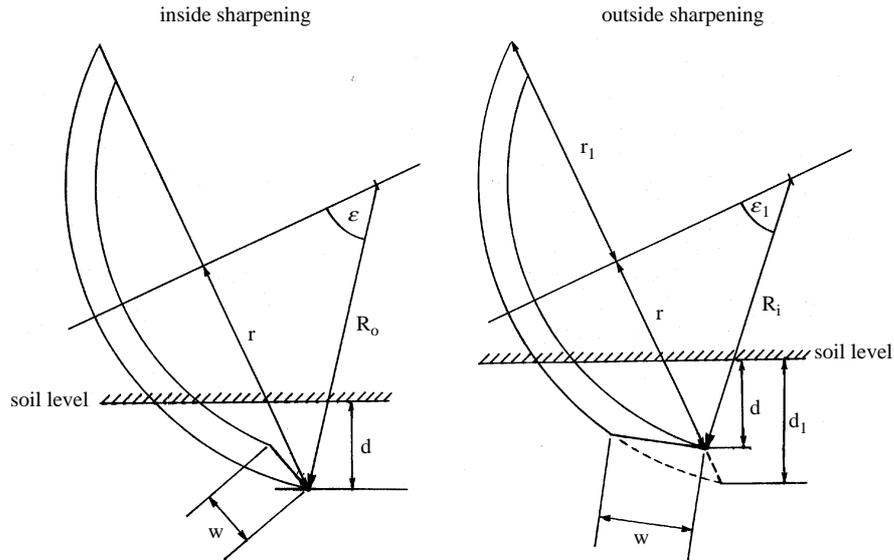
Fig. 14. Geometrical parameters for inside and outside sharpened discs
