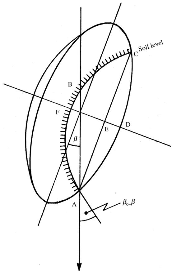
*Fig. 2. Bearing and pressure areas of a disc at an angle  $\beta$  to the direction of motion projected on to a horizontal plane ( $A_{bh} = AFB$ ;  $A'_{ph} = AFBC$ ;  $A_c = AECD$ )*
