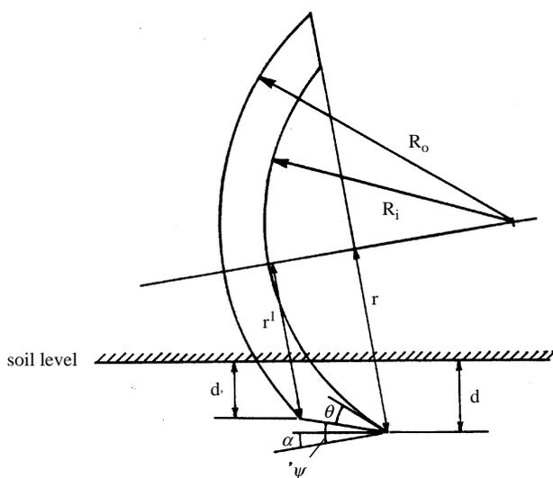
Fig. 15. Geometrical parameters and clearance angles for an outside sharpened disc
