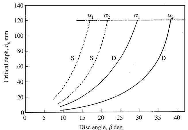
Fig. 7. Variation of critical depth ( $d_c$ ) with disc angle ( $\beta$ ) for 85 mm disc concavity (D) and 51 mm disc concavity (S) (tilt angles;  $\alpha_1 = 10^\circ$ ;  $\alpha_2 = 30^\circ$ ; curves intersect the working depth line at the critical angle)
