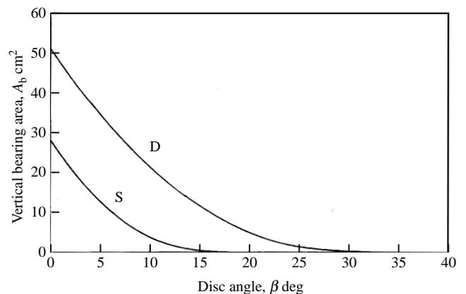
Fig. 9. Variation of vertical bearing area ( $A_b$ ) with disc angle ( $\beta$ ) at a working depth of 120 mm and a tilt angle  $\alpha = 20^\circ$  [disc concavity: 51 mm (S); 85 mm (D)]
