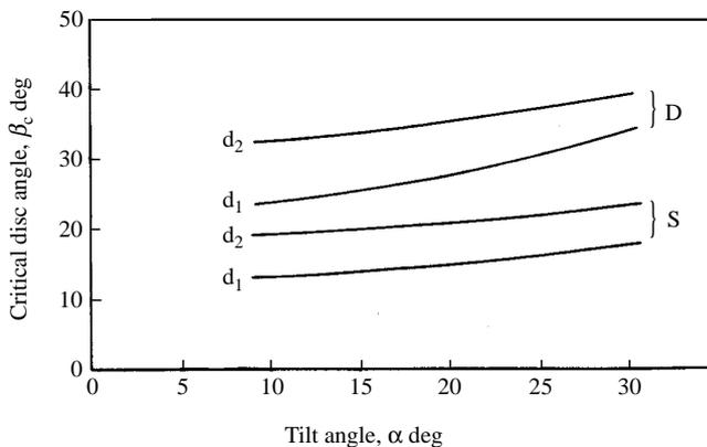
Fig. 6. Variation of critical disc angle ( $\beta_c$ ) with tilt angle ( $\alpha$ ) for 85 mm disc concavity (D) and 51 mm disc concavity (S) (working depths:  $d_1 = 60$  mm;  $d_2 = 180$  mm)
