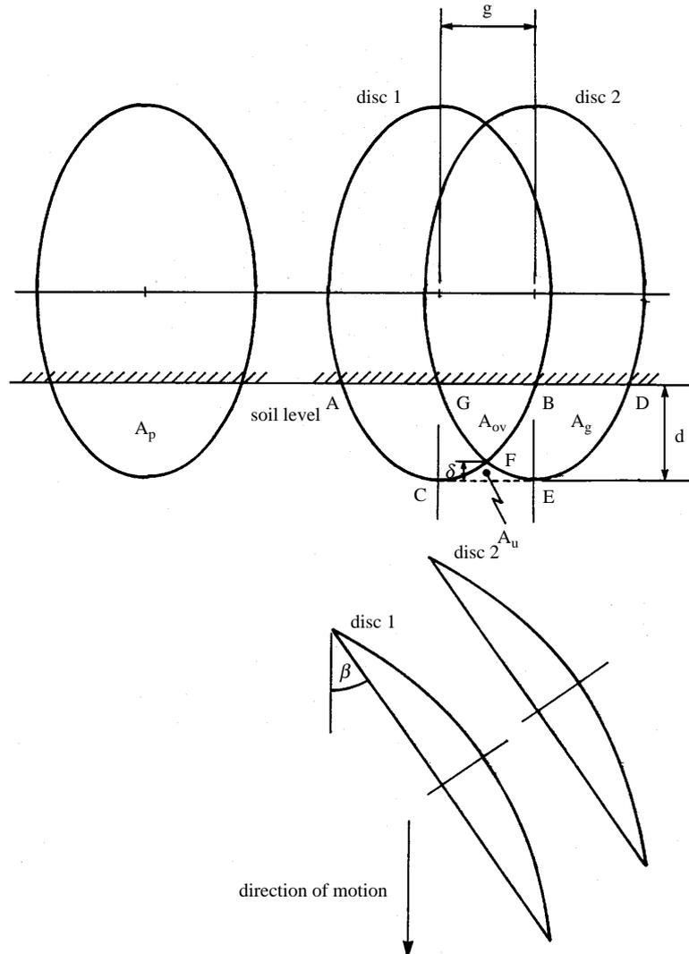
Fig. 4. Pressure areas and area of uncut soil of discs in a gang projected on to a vertical plane for  $\alpha = 0^\circ$  (upper: elevation; lower: plan;  $A_p = ACFB = DEFG$ ;  $A_{ov} = BFG$ ;  $A_g = BFG$ ;  $A_u = CFE$ )
