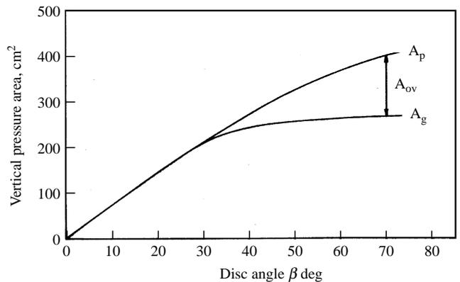
Fig. 12. Variation of vertical pressure areas ( $A_p$ ,  $A_g$  and  $A_{ov}$ ) with disc angle ( $\beta$ ) for ganged discs at a working depth of 120 mm and a tilt angle  $\alpha = 20^\circ$  (disc concavity = 51 mm and disc spacing = 240 mm) ( $A_p$ : vertical pressure area;  $A_{ov}$ : overlap area;  $A_g$ : area cut by an individual disc)
