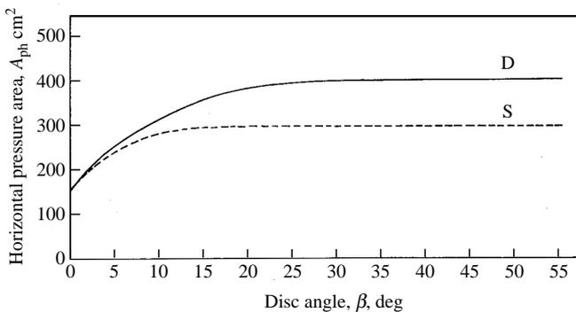
Fig. 10. Variation of horizontal pressure area ( $A_{ph}$ ) with disc angle ( $\beta$ ) at a working depth of 120 mm and a tilt angle  $\alpha = 20^\circ$  [disc concavity: 51 mm (S); 85 mm (D)]
