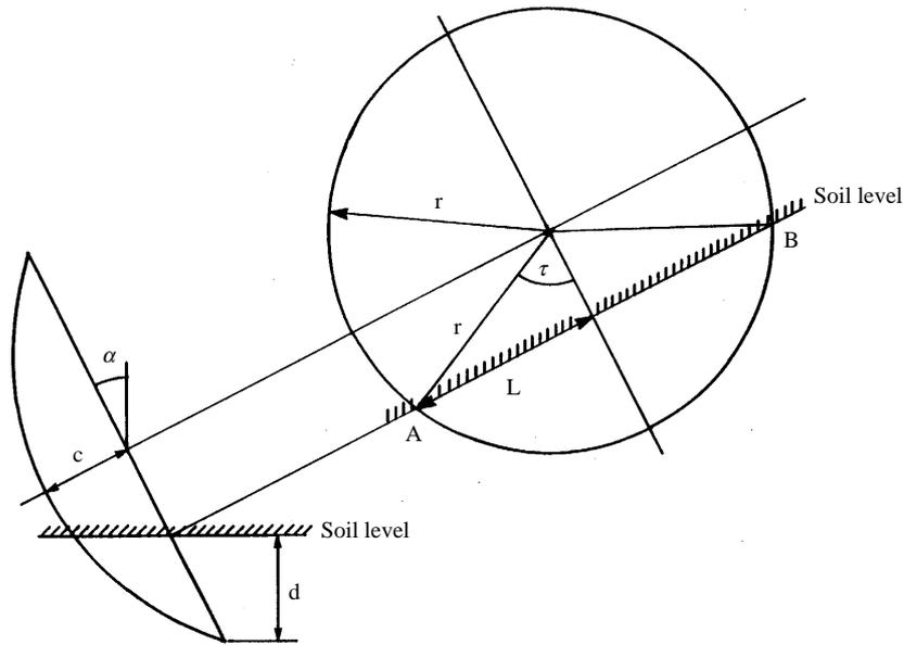
Fig. 5. Chord of intersection AB ( $=2L$ ) of soil surface with disc circular edge for a disc inclined at an angle  $\alpha$  to the vertical
