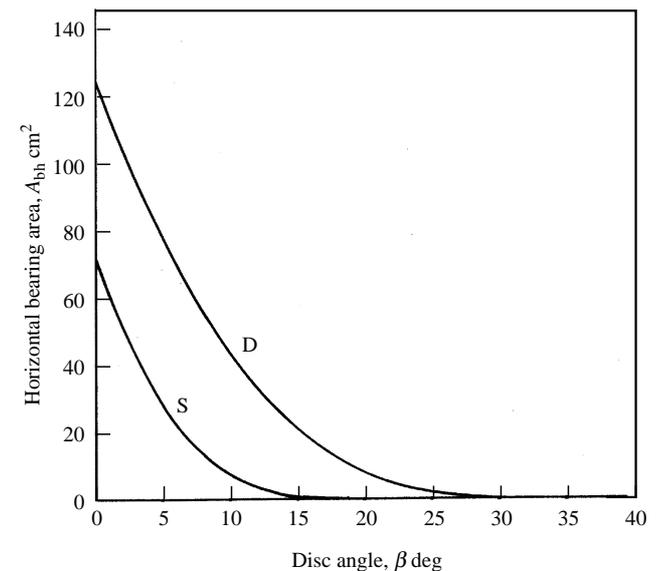
Fig. 11. Variation of horizontal bearing area ( $A_{bh}$ ) with disc angle ( $\beta$ ) at a working depth of 120 mm and a tilt angle  $\alpha = 20^\circ$  [disc concavity: 51 mm (S); 85 mm (D)]
