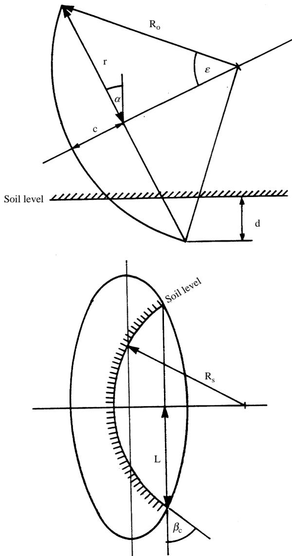
*Fig. 1. Geometrical parameters of a disc tilted at an angle  $\alpha$  to the vertical plane (upper: elevation; lower: plan)*
