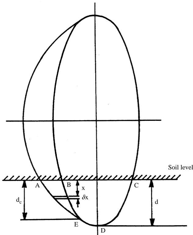
Fig. 3. Bearing and pressure areas of a disc projected on to a vertical plane ( $A_b = ABE$ ;  $A_p = BCDE$ )
