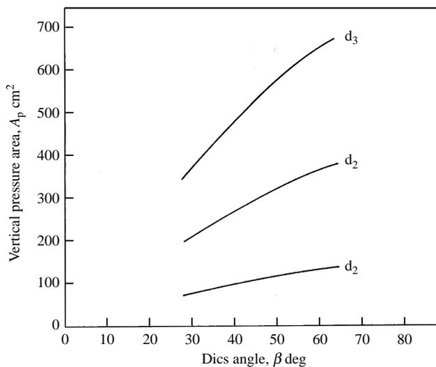
Fig. 8. Variation of vertical pressure area ( $A_p$ ) with disc angle ( $\beta$ ) for 51 mm disc concavity at a tilt angle  $\alpha = 20^\circ$  (working depths;  $d_1 = 60$  mm;  $d_2 = 120$  mm;  $d_3 = 180$  mm)
