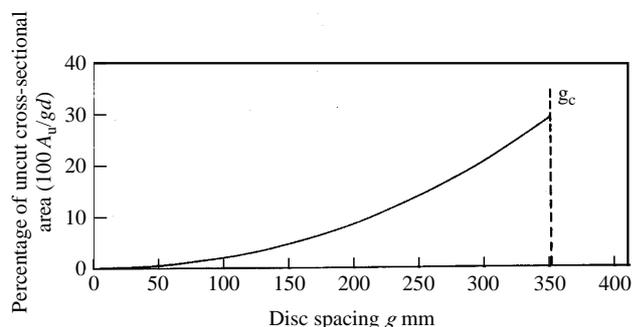
Fig. 13. Variation of the percentage of uncut soil cross-sectional area between adjacent discs in a gang with disc spacing ( $g$ ) for a 51 mm disc concavity (working depth = 120 mm; tilt angle  $\alpha = 20^\circ$ ; disc angle  $\beta = 45^\circ$ ; critical spacing  $g_c = 35.1$  mm)
