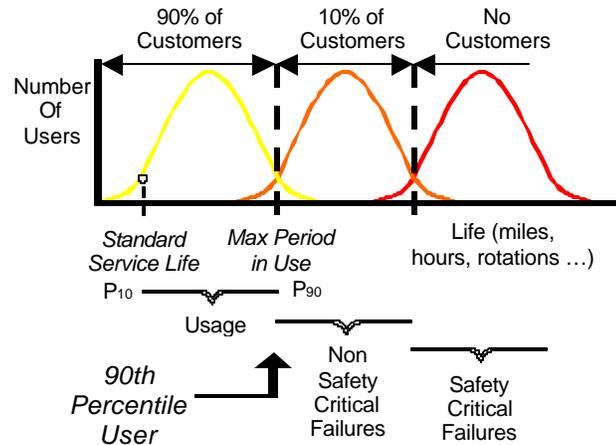
**Figure 15. Durability Targets for 90th Percentile Customer.**
