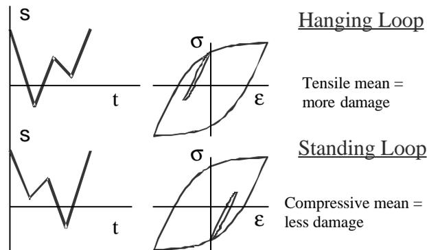
Figure 6. Illustration showing the effect of cycle sequence.
