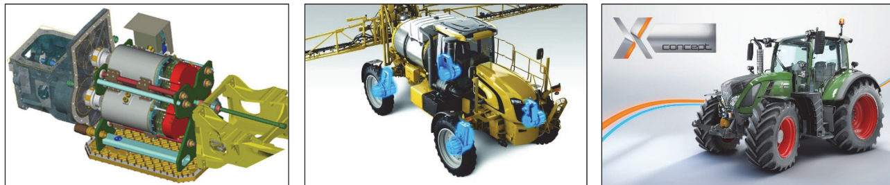
Figure 2. MELA, electric tractor transmission system, 2004 (left); eRoGator, electric sprayer with wheel-hub drives, 2010 (middle); Fendt X Concept, electrified tractor with 130 kW power generator, 2013 (right).
