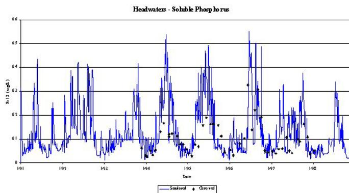
**Figure 2: Observed and Simulated Soluble Phosphorous in Deep Creek**
