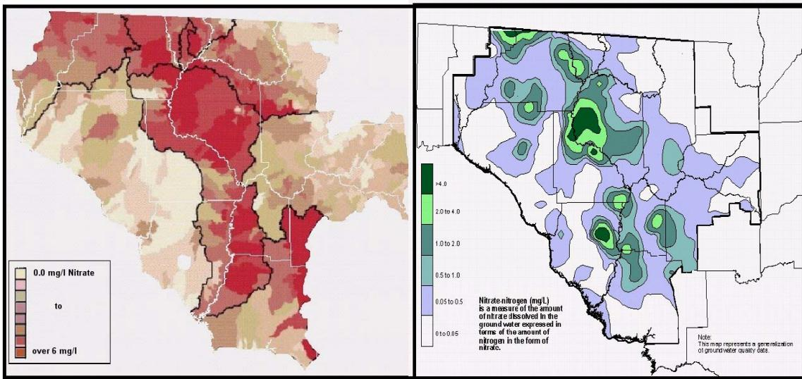
**Figure 1: Observed (left) and Simulated (right) Groundwater Nitrate Levels in the Suwannee River Basin**
