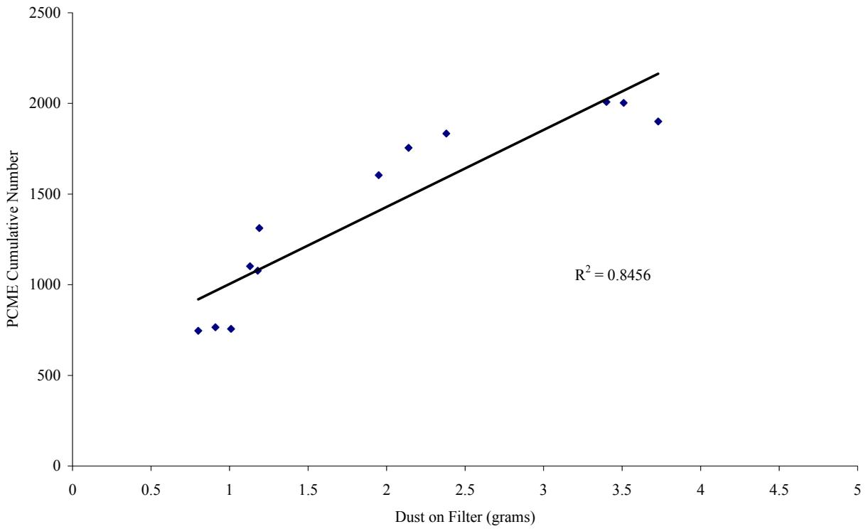
**Figure 2. Comparison of PCME data to filter catch for 0.31 m (12 inch) cyclone.**
