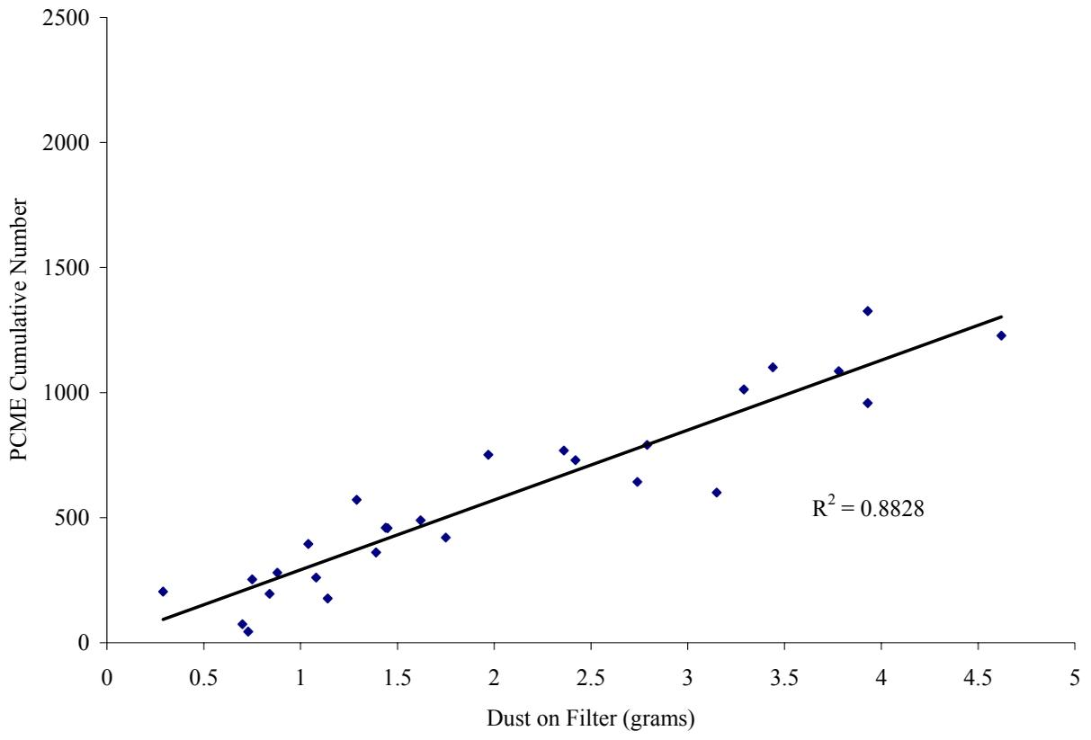
**Figure 3. Comparison of PCME data to filter catch for 0.43 m (17 inch) cyclones.**
