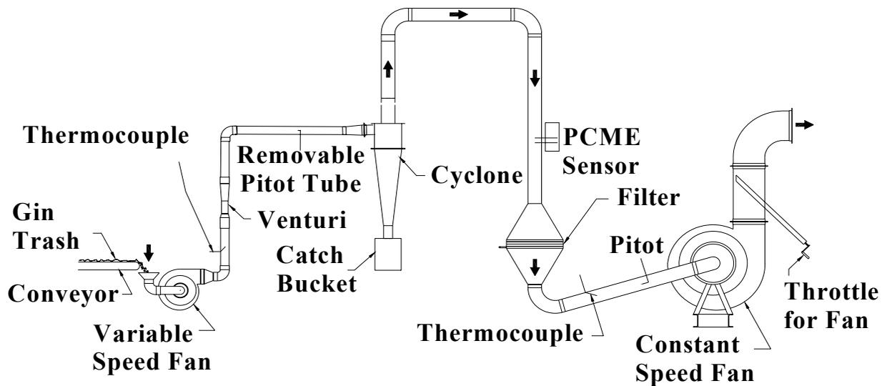
**Figure 1. Configuration of equipment used to evaluate PCME device. System hardware and test methods remained the same for both cyclone sizes.**
