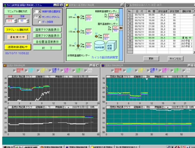
Figure 3. Temperature and humidity control program.
