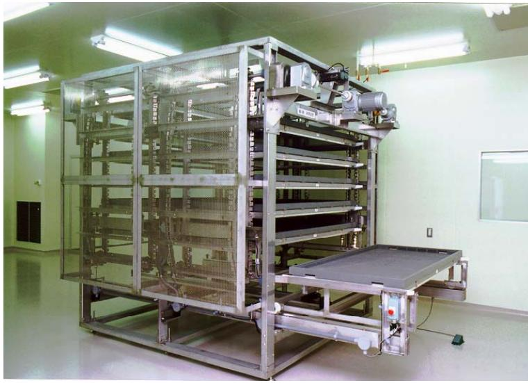
**Figure 4. Automatic silkworm rearing system.**
