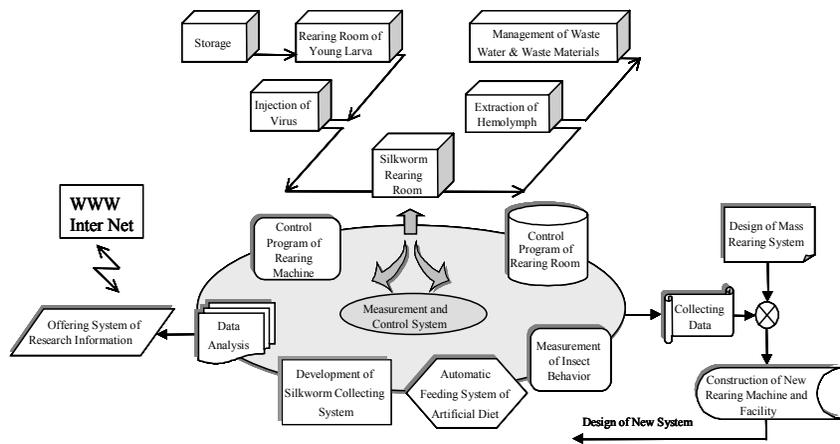
Figure 1. Schematic diagram of insect factory.
