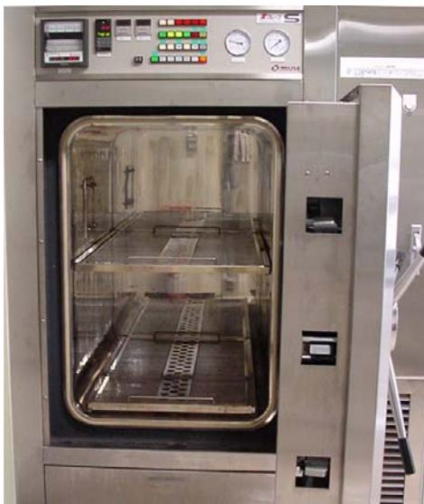
**Figure 5. View of Autoclave used on waste materials.**
