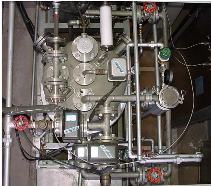
**Figure 8. High temperature pressure type steam sterilizer.**
