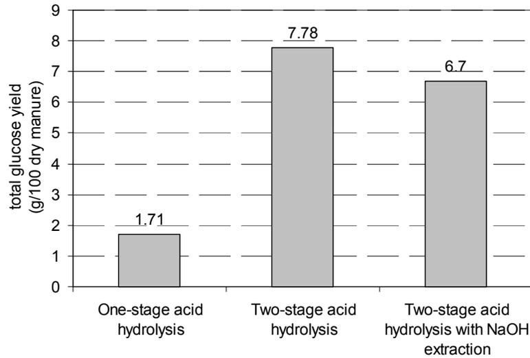
**Figure 3. Comparison of total glucose yields of different hydrolysis**
