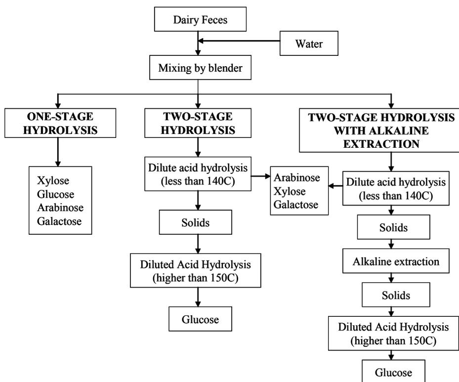
Figure 1. Procedure of acid hydrolysis of dairy manure
