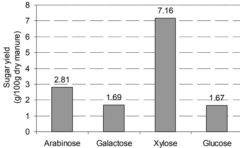
**Figure 2. Individual sugar yields at the optimal condition of one-stage hydrolysis**
