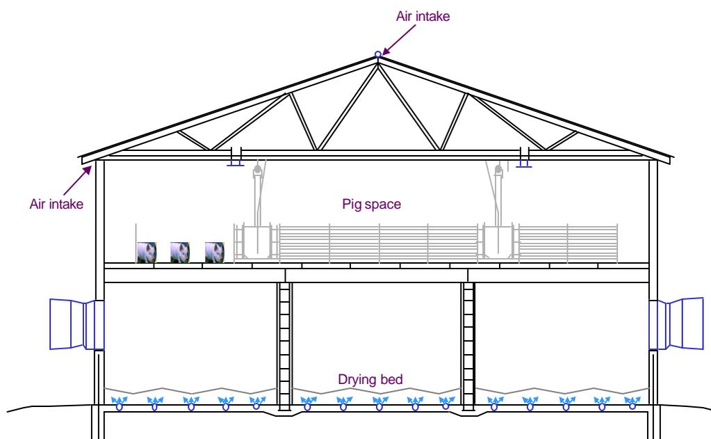
Figure 7. Cross-section view of commercial version of High-Rise™ finishing facility.
