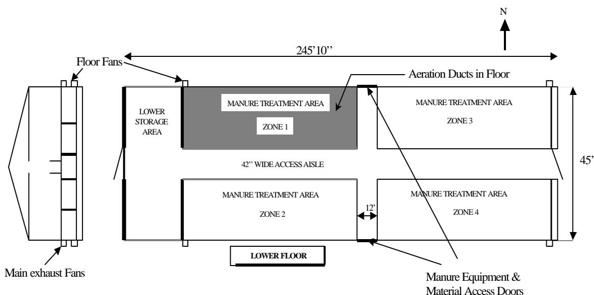
Figure 2. Schematic of lower-story floor for the 4-M Farms High-Rise™ Hog Building with drying zones identified.
