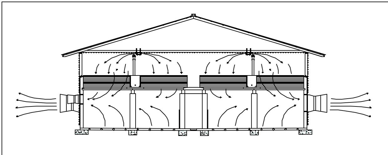
Figure 3. Design airflow patterns within a High-Rise™ swine finishing facility (4M Farms research /demonstration facility).
