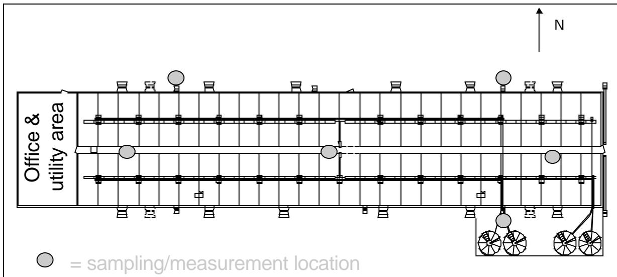
Figure 4. Gas measurement locations on a plan view of research / demonstration facility.
