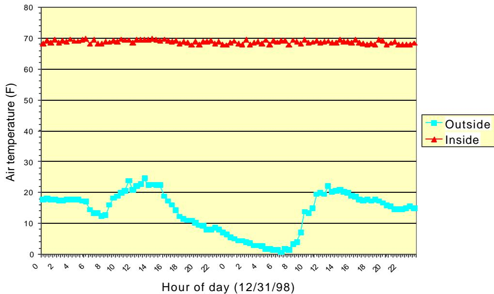
Figure 5. Mean air temperature in the pig space of the High-Rise™ finishing facility compared to outdoor temperature during a representative period of cold weather.
