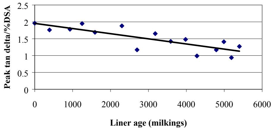
**Figure 10** Change in tan delta with strain as liners age.
