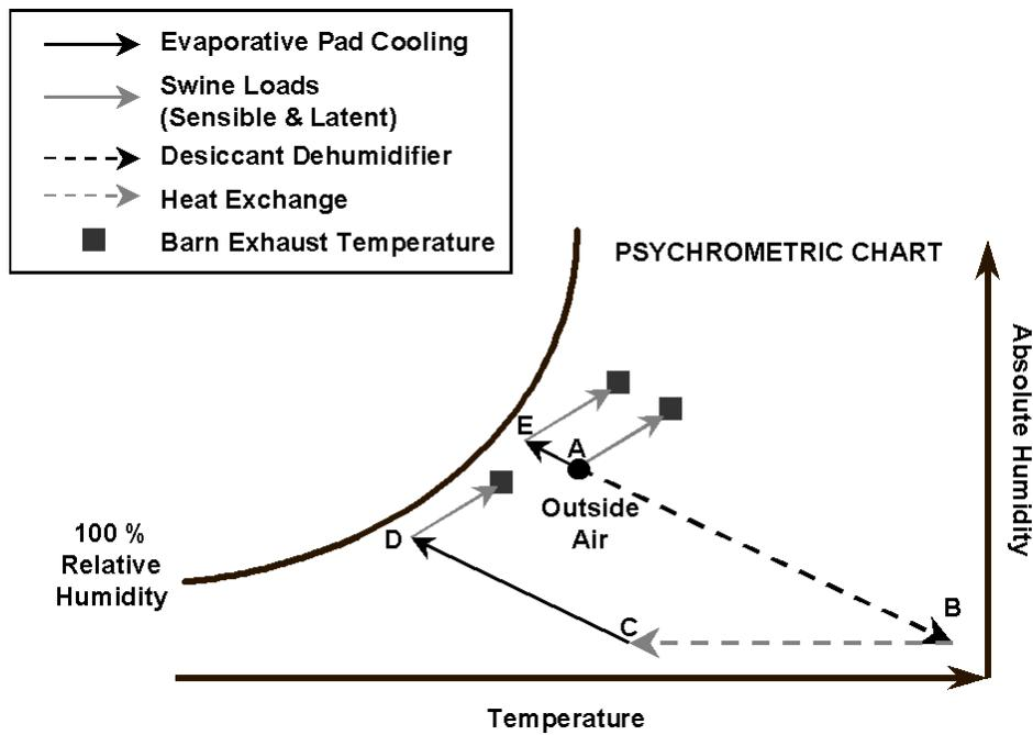
Figure 2. Psychrometric chart plotting the operational conditions for a desiccant-based system using an evaporative pad. Each path between points in the chart is as follows: Path A-B: outside air passes through the desiccant wheel; Path B-C: sensible heat recovery from heat exchange wheel; Path C-D: evaporative pad cooling.
