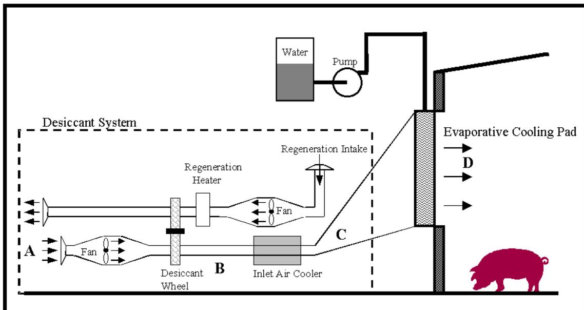
Figure 3. Design concept for swine facility desiccant system with evaporative cooling pad.
