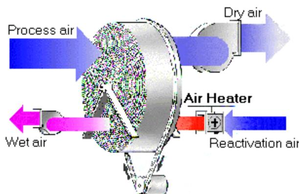
Figure 1. Schematic of desiccant wheel operation including process and reactivation air streams.
