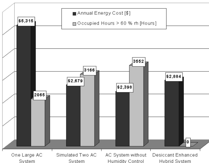
Figure 4. Simulation performance results for AC cooling systems compared to desiccant system.
