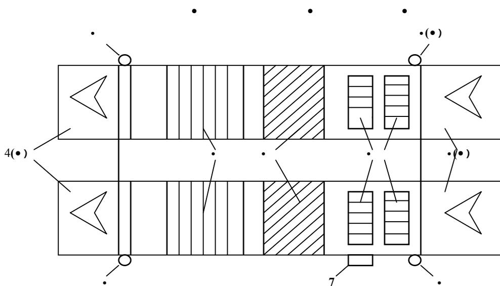
1.Roller 2.Axle weight test platform 3. Braking torque test platform 4•6.Guide deck
