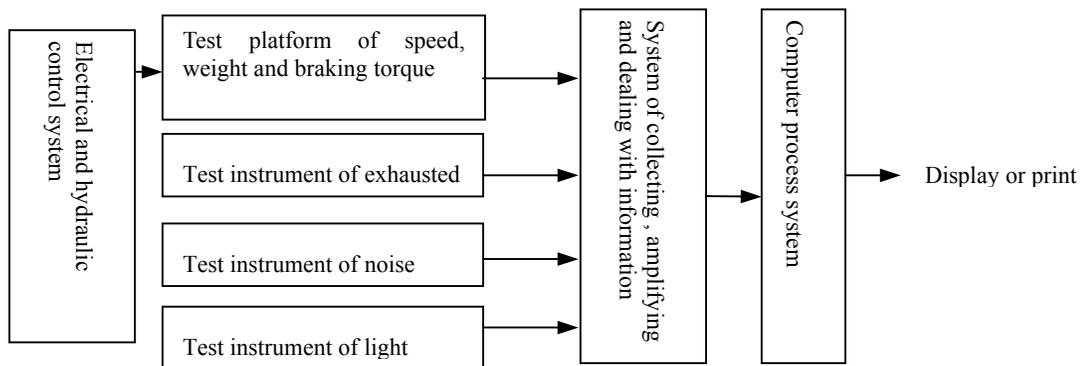
**Figure 1 Structure and principle of the test equipment**
