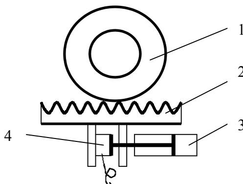
1.Wheel 2. Movement deck 3. Hydraulic cylinder 4 Sensor
