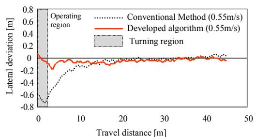
Figure 8. Comparison between developed switch-back turning and conventional one
