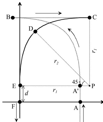
Figure 3. Algorithm of path creation for switch-back turning in case of left turning
