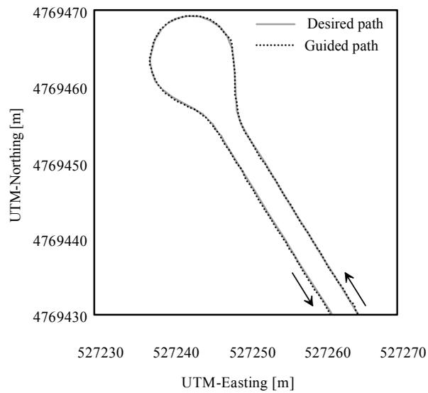
Figure 6. Guided path and desired path of forward turning at 1.3 m/s
