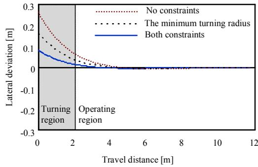
Figure 5. Comparison of turning accuracy by applying different constraints on simulation of forward turning
