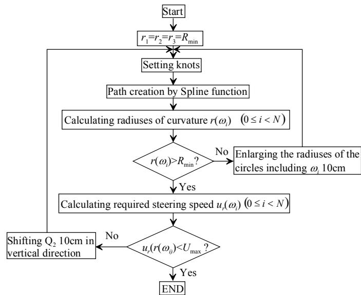
Figure 2. Flowchart of path creation of forward turning
