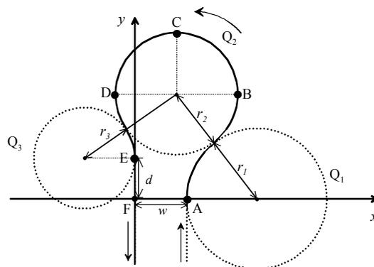
Figure 1. Algorithm of path creation for forward turning in case of left turning
