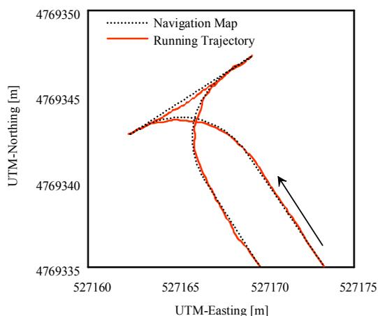
Figure 7. Guided path and desired path of switch-back turning at 1.3 m/s
