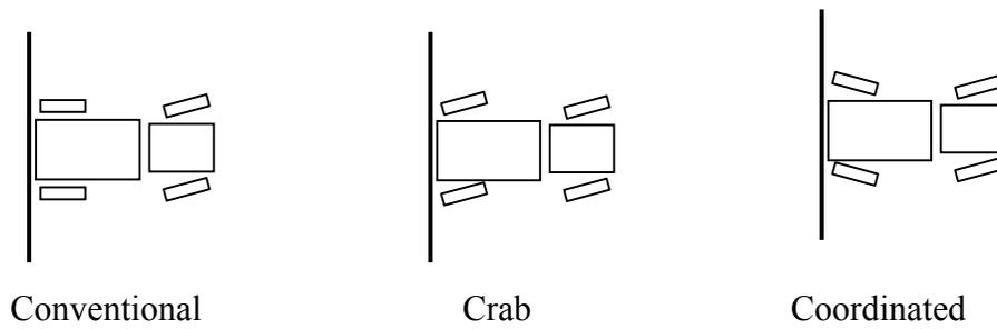
Figure 1. With four-wheel steering, three modes of steering exist: conventional, crab and coordinated.
