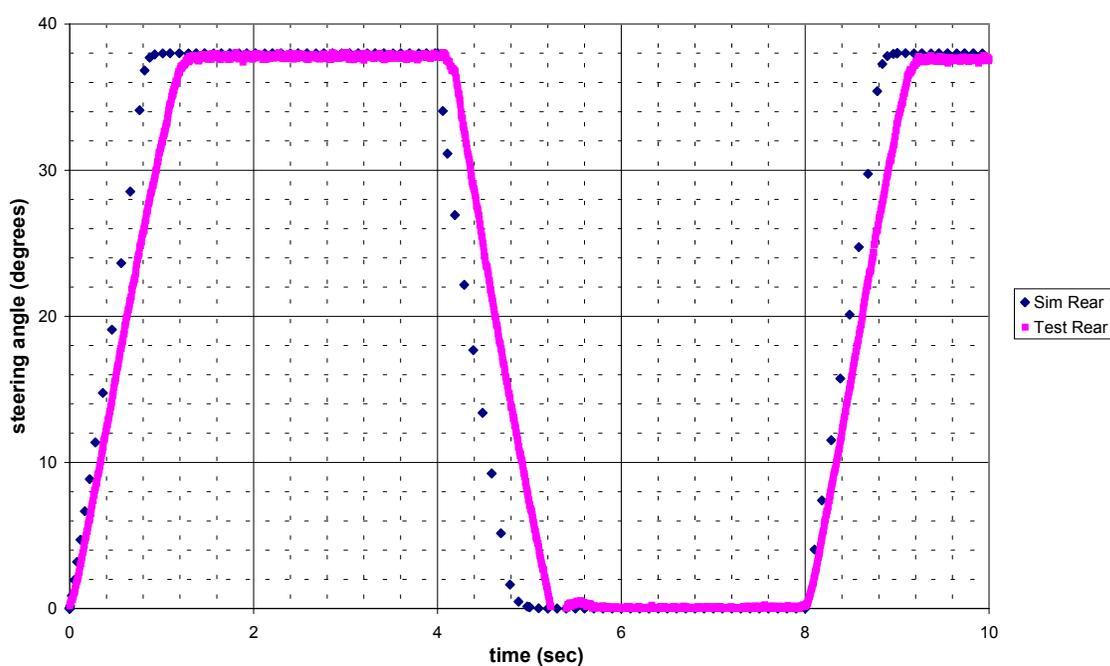
Figure 6. Plot of simulated steering response of wheels to step input in steering angle assuming full flow through valves and plot of actual wheel response on vehicle.
