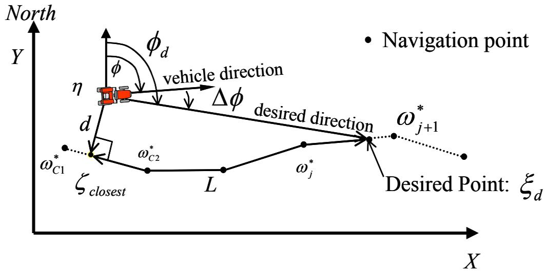
Figure 5. Definition of navigation signals based on map.
