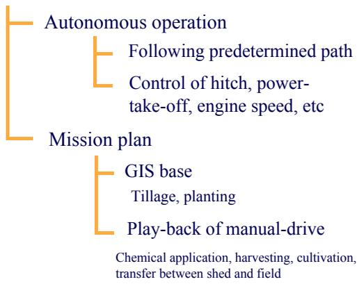
Figure 2. Functioning of a robot tractor.
