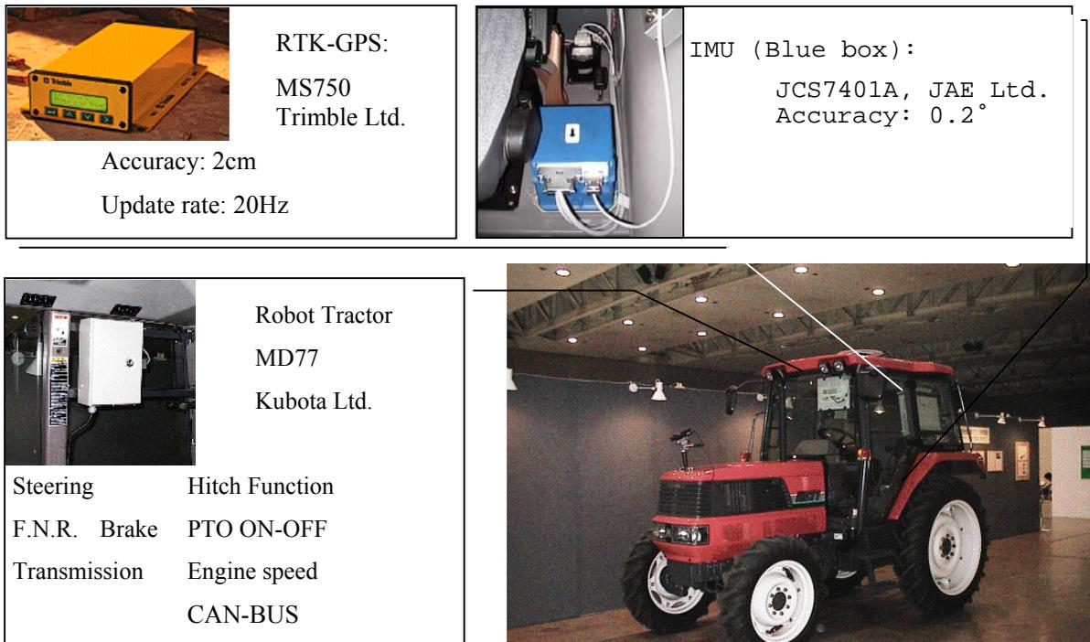
Figure 1. Robot tractor hardware
