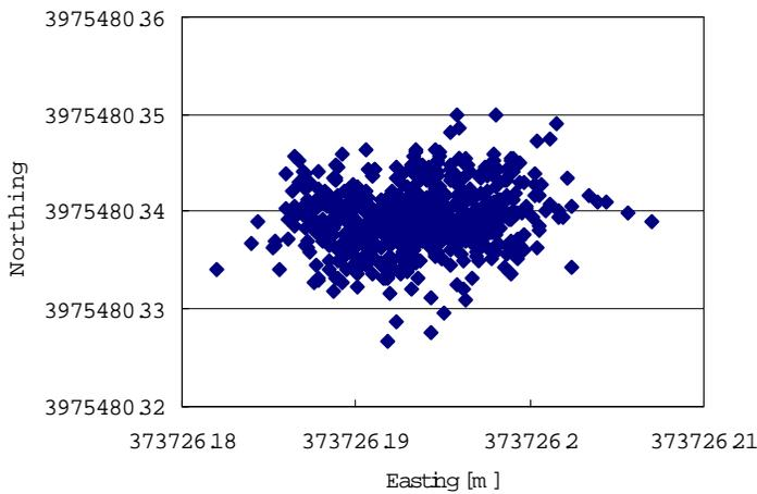
Figure 3. Accuracy of the tested RTK-GPS
