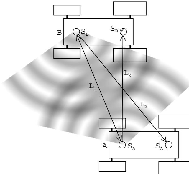
Figure 1. Schematic diagram of the proposed relative position detection system using diffuse light
