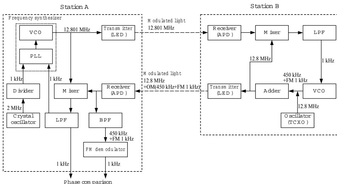
Figure 4. Block diagram of the developed range finder
