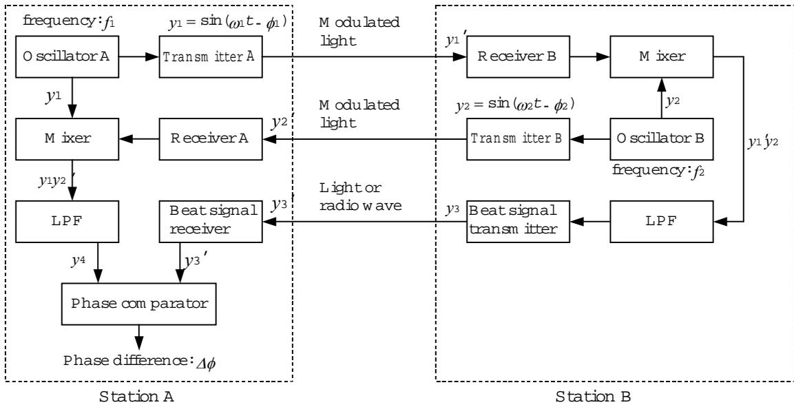
Figure 2. Principle of the developed range-finder
