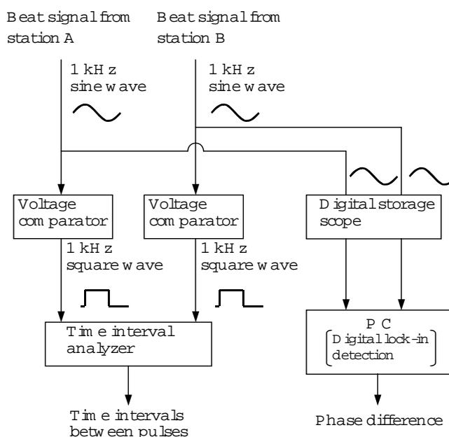
Figure 5. Schematic diagram of the phase difference measurements
