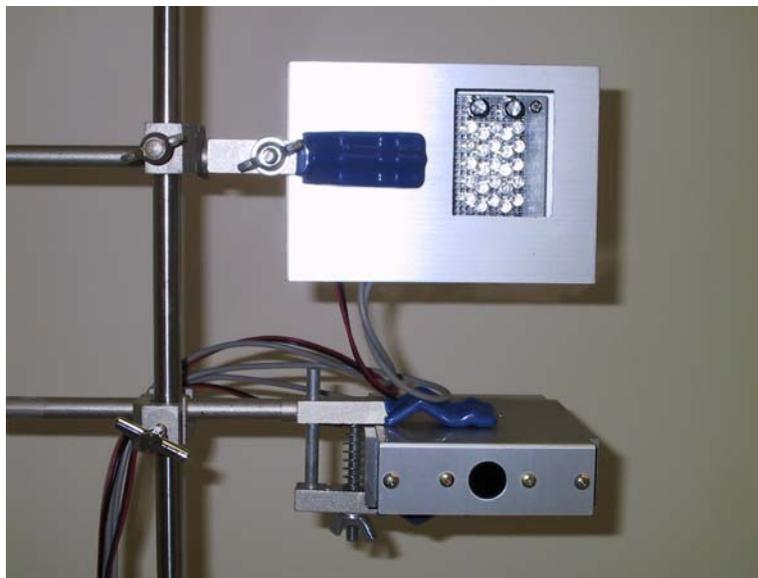
Figure 3. Optical transmitter and receiver
