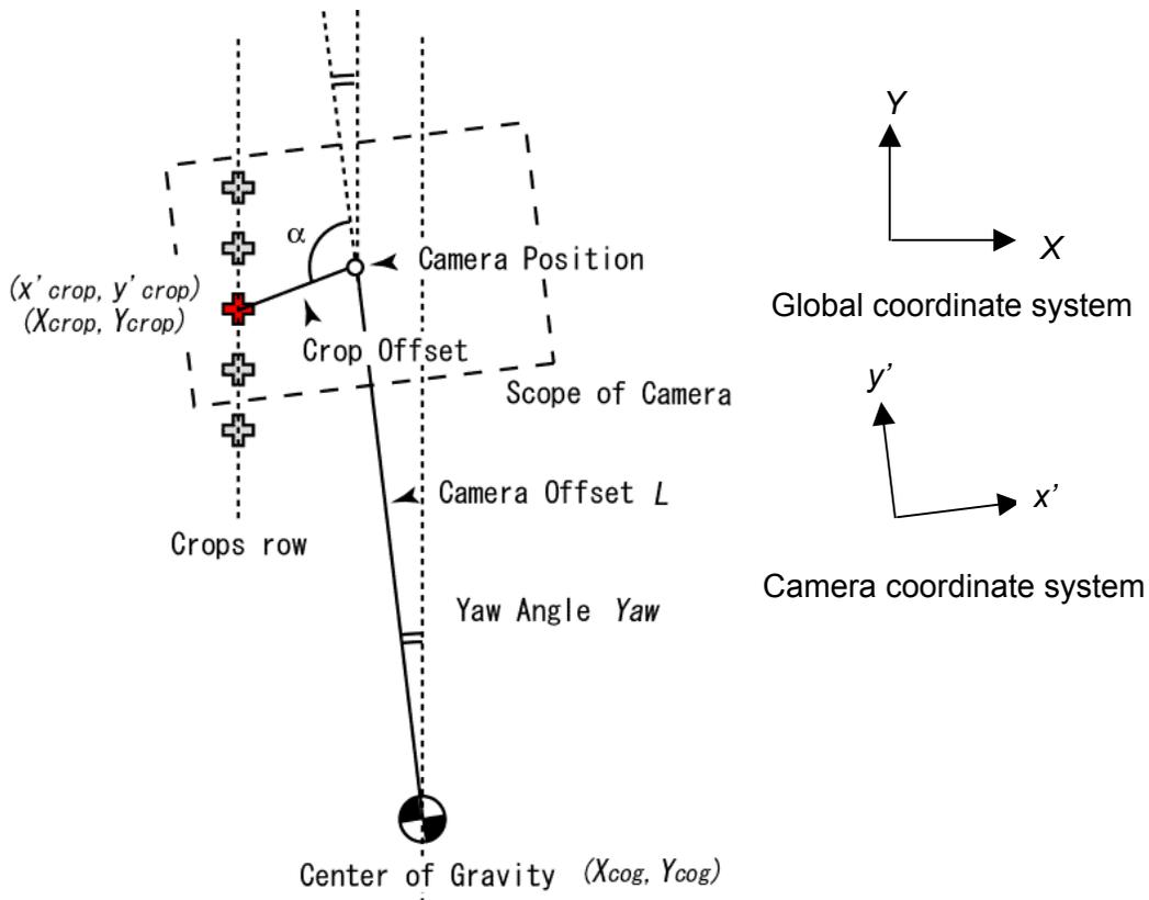
Figure 6. Camera and Global coordinate systems.
