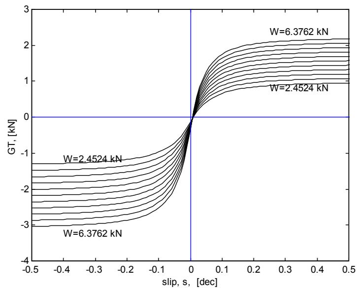
Fig. 2. Gross traction force of a driven wheel for various vertical loads.
