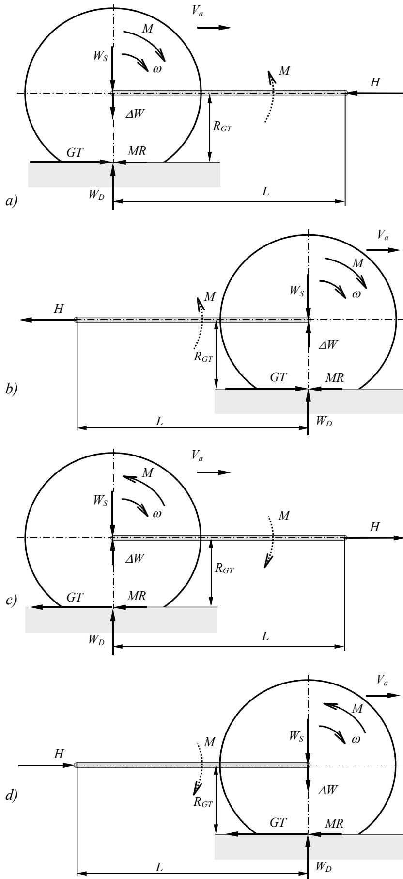
Fig. 3. Influence of load transfer on a driven wheel: a) rear wheel in driving mode; b) front wheel in driving mode; c) rear pulled wheel; d) front pushed wheel.
