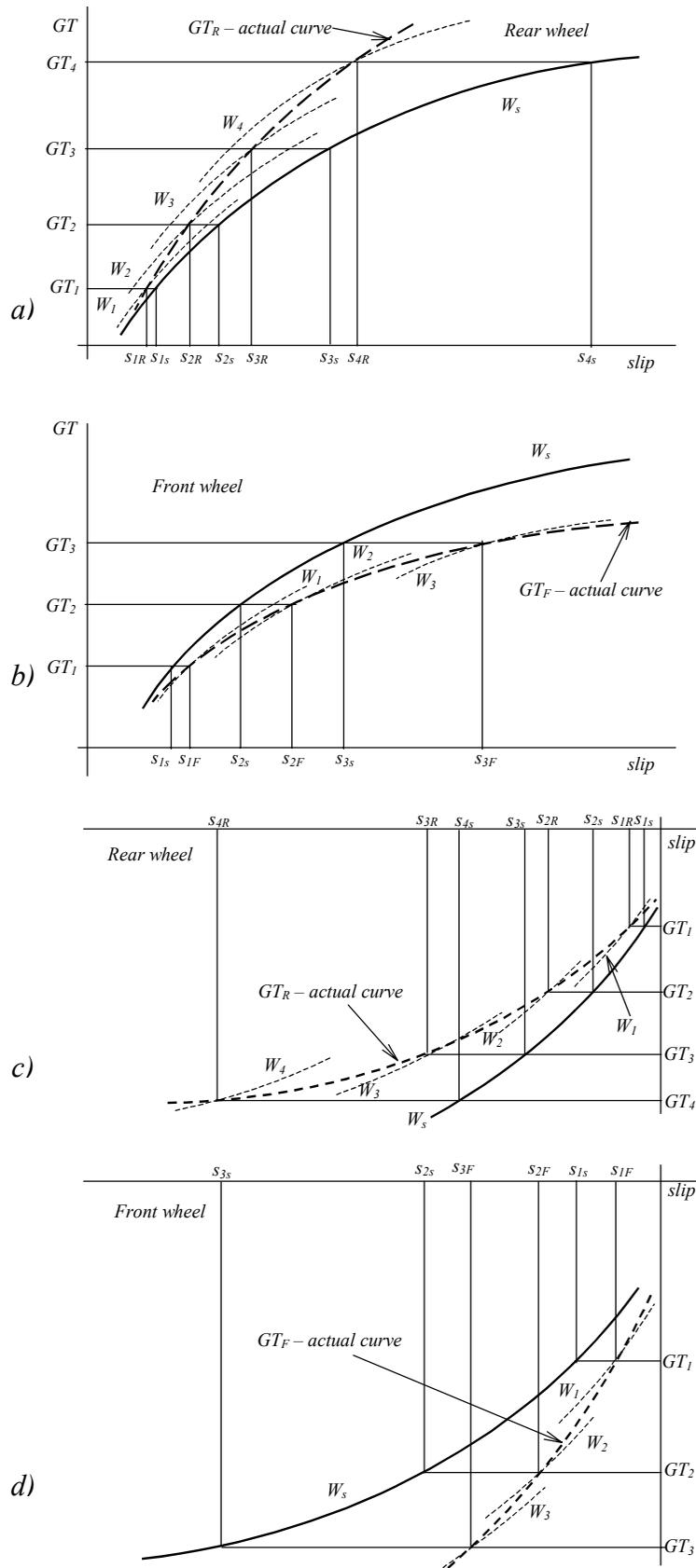
Fig. 4. Traction performance of a driven wheel affected by load transfer: a) rear wheel in driving mode; b) front wheel in driving mode; c) rear pulled wheel; d) front pushed wheel.
