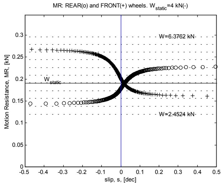
Fig. 6. Motion resistance simulations of front and rear driven wheels.
