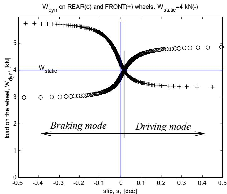
Fig. 5. Simulations of vertical load on the driven wheel vs. slip.
