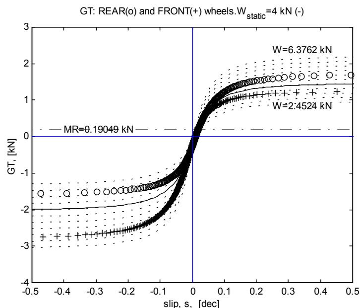
Fig. 7. Gross traction force simulations of front and rear driven wheels
