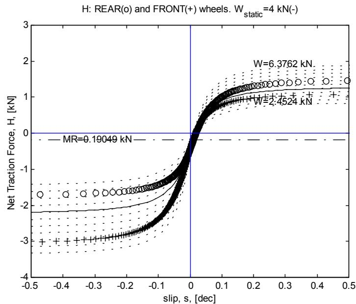
Fig. 8. Net traction force simulations of front and rear driven wheels.
