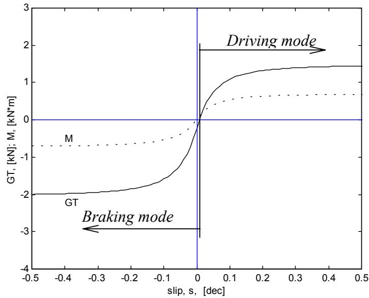
Fig. 1. Traction performance of a driven wheel ( $W_{static} = 4.0 \text{ kN}$ ).
